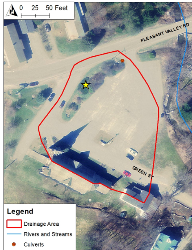
Figure 19. Runoff from the St. Thomas Church Parking Lot drainage area, shown in red, is proposed to be directed to a bioretention shown with a star.
